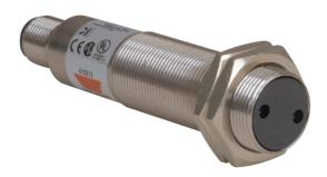
PA Series Diffuse-reflective Photoelectric Sensor, modulated infrared light M18 nickel-plated brass housing, 20 to 250V AC power supply, 500mA SCR NC output, 400mm sensing range, IP67 rating, M12 plug 2m pre-wired cable
